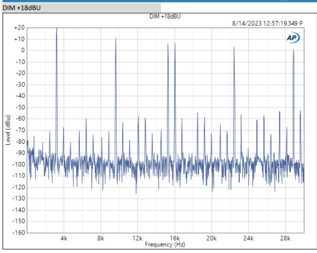
Another DIM test, this time at +18dBU out. This, like other high level tests, are intended to illustrate how well the DUT handles high level, complex signals.
