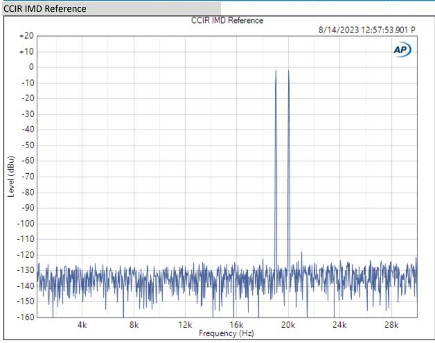
This FFT graph is an example of what the next 2 graphs would look like with a perfect system. The two signals, one each at 19kHz and 20kHz are mixed together in the DUT. Intermodulation Distortion will present at signals at 1kHz (the difference between 19 and 20kHz) across the frequency band.
