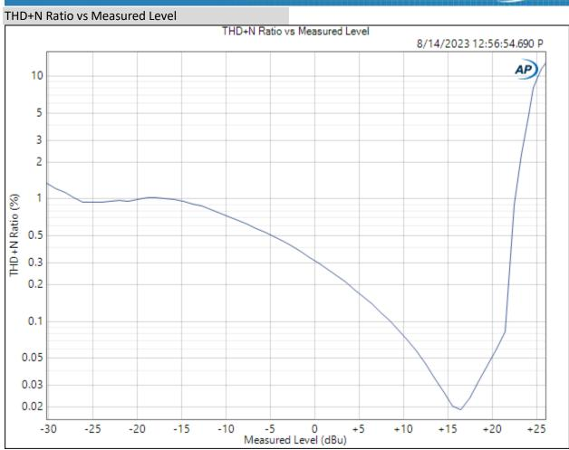
This graph shows THD+N as the input level increases. The measurement shown on the horizontal axis is the output level of the Device Under Test (DUT).
