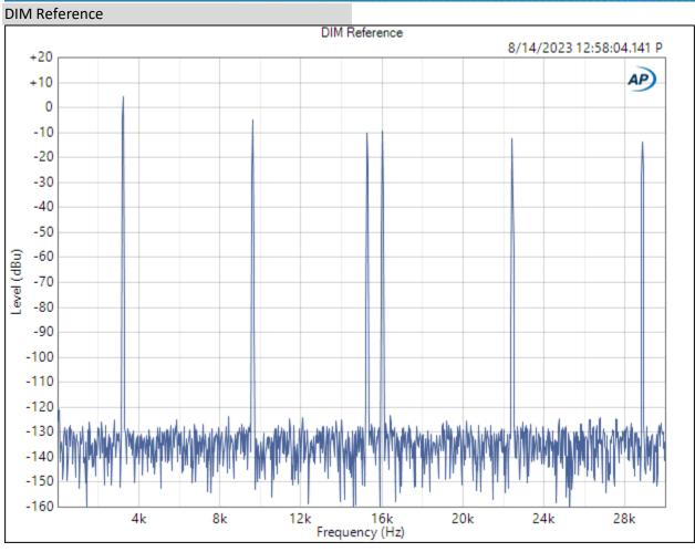
Dynamic Intermodulation Distortion (DIM) is a relatively new measurement performed with a 3kHz square wave modulated by a 15kHz sine wave.
