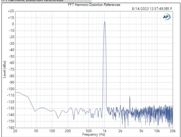
This Fast Fourier Tranform (FFT) graph shows what a perfect device would look like in the next two tests. Vertical shows level, horizontal frequency. A 1kHz signal is present as shown by the narrow vertical column at 1kHz and there is a very minor harmonic at 3kHz, down >114dB from the signal and no other harmonics. Use this as a baseline for reviewing the next two graphs.
