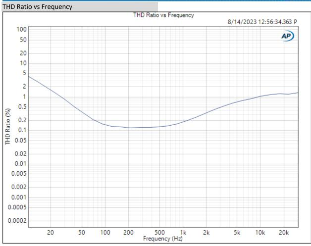
This graph shows Total Harmonic Distortion for each frequency from 10Hz to 30kHz at 40dB of gain. Most measurements of THD include noise, this measurement is THD only to display harmonic distortion more accurately.
