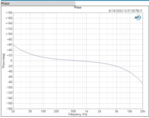
Phase shift measurements show the change in phase at each frequency measured. Significant shifts in phase can color the sound. A perfect reading would be a flat line at 0 degrees.
