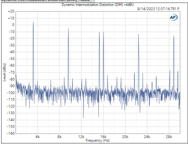
Any extra peaks, beyond the example above, indicate the DUT is not handling complex signals well.
