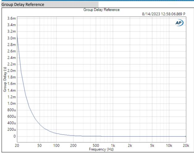
This shows the equipment baseline for Group Delay. Unfortunately, the Audio Precision doesn't provide a perfectly flat Group Delay measurement in the very low frequencies, so you need to compare the delay in this graph with the other to understand the performance.
