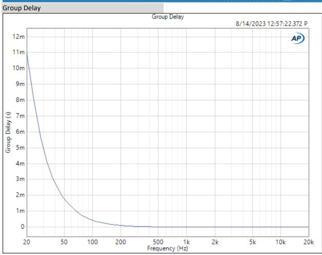
Group delay is intended to show the time offset between input and output. It measures, in milliseconds, the delay at each measured frequency. Significant changes in Group Delay can alter how a complex signal passes through the device. If treble is delayed by 50-100 ms vs low frequencies, this can alter how the mix sounds.
