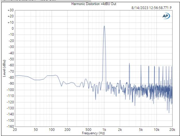
This graph displays the spectrum with a 1kHz tone at +4dBU out.
