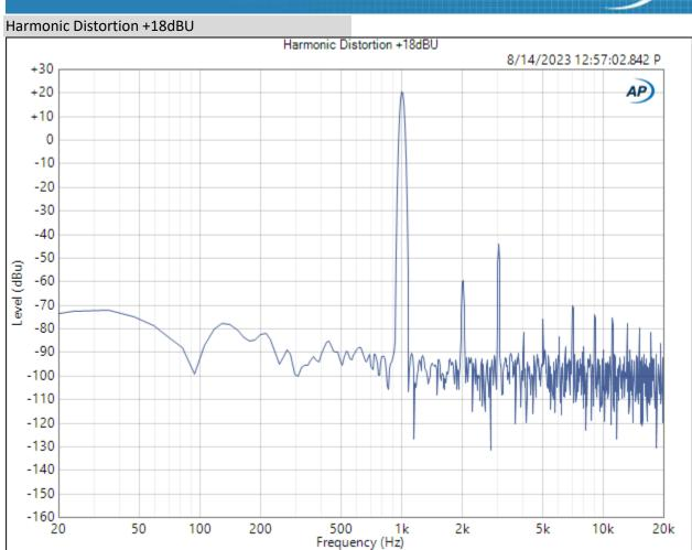
This chart displays the spectrum with a 1kHz tone at +18dBU out. Examine any differences between this and the previous chart to see if the signal degrades with increasing level.
